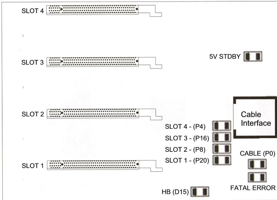
**Xpander is functioning properly once the Cable (P0) LED lights green.**
