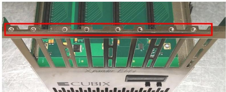
11. Install the graphics or other controller(s) in the Xpander PCIe slot(s) and connect PCIe auxiliary power cables (see the image at the right). Desktop Elite with a 1200Watt provides four sets of aux power connectors with 8P + 6P. Optional 8P + 8P aux power connectors are available. Seat each set of connectors properly in the GPU devices so the host computer system and operating system (OS) can detect and use the devices.
