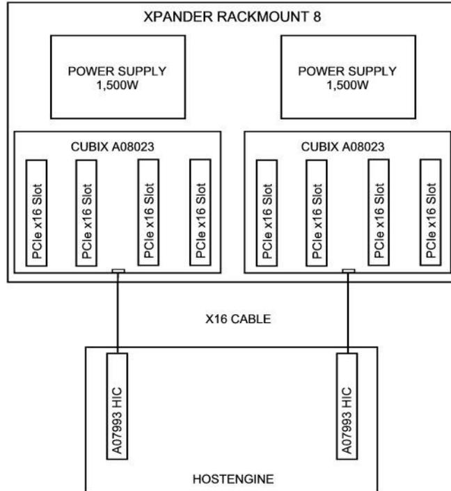
By connecting HostEngine to GPU-Xpander Rackmount 8, you can add eight double-wide GPUs such as NVIDIA® Quadro M5000 or M6000 to the HostEngine 2U computer for running Autodesk® 3ds Max or Bunspeed® Shot with Mental
