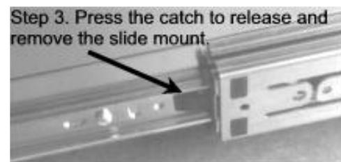
**Step 3. Press the catch to release and remove the slide mount.**
