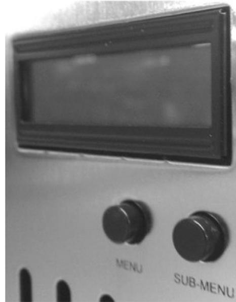
When a fault occurs, the LCD will jump to that fault and the LCD backlight will flash on / off. Press the left button to acknowledge the fault and the LCD will stop flashing and enable normal operation. The LCD will continue to display the fault at the applicable sub-menu until you clear the fault.
