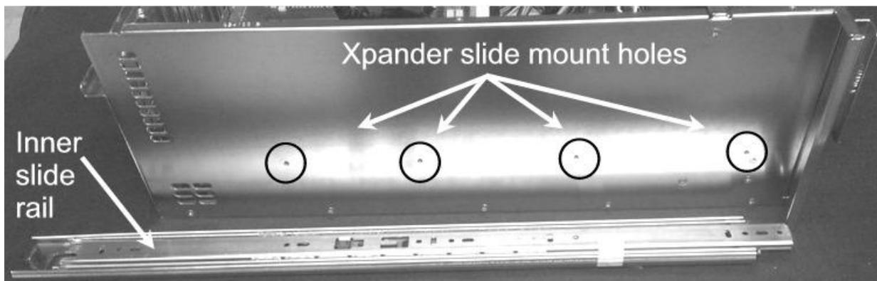
3. Remove the inner slide rail, or slide mount, from the outer rail and mount it to Xpander using the Xpander slide mounting holes. To release each outer slide mount, slide it toward the rear of the enclosure until it stops. Press the catch to release and remove the outer slide mount as you can see in the image at the right.
