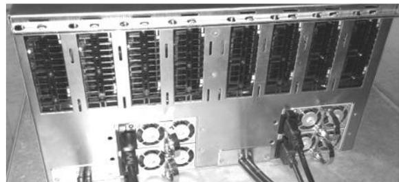
Remove both AC power cords from the power modules connected to the main board, or MIB, in which you install GPUs.
