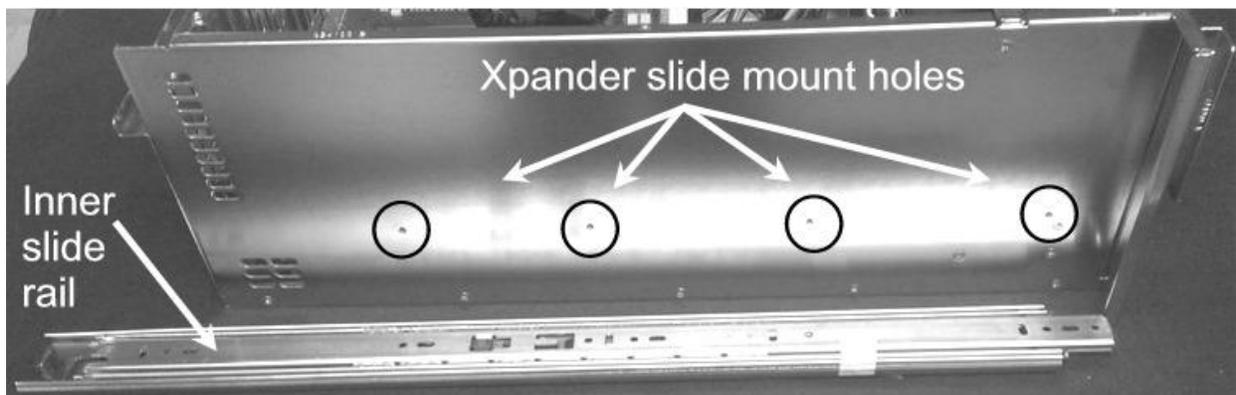
3. Remove the inner slide rail, or slide mount, from the outer rail and mount it to Xpander using the Xpander slide mounting holes. To release each outer slide mount, slide it toward the rear of the enclosure until it stops. Press the catch to release and remove the
