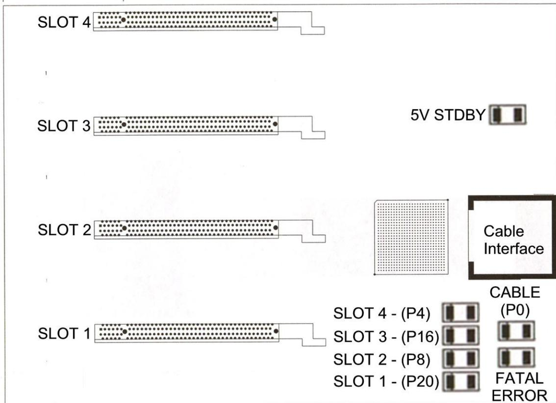
**Xpander MIBs are functioning properly once each Cable LED (P0) lights green. Proceed to the next step to install adapters.**
