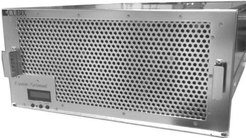
Rack Mount 8 provides two Main Interface Boards (MIBs) connected to each of one or two host computers with a PCIe x16 cable and four PCIe x16 slots for a total of eight double-wide GPUs like NVIDIA GTX TITAN X / 980. Each MIB connects via a PCIe x16 cable to a HIC in a host computer. Connect each MIB to one of two HICs in one host or each MIB to a HIC in each of two host computers. Each MIB inside Rack Mount 8 connects to one host computer.
