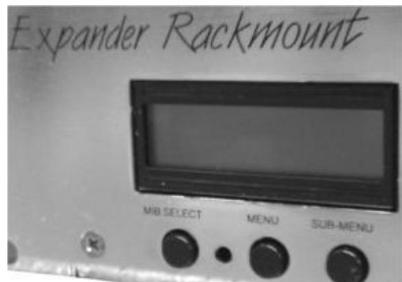
by pressing the left button for a MIB, the middle button for a menu selection and then the right button for a sub-menu selection.
