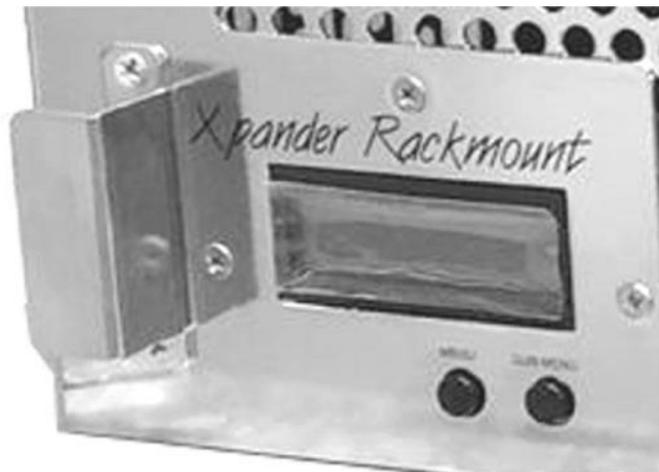
The upper right corner of the LCD shows a flashing asterisk \*. This indicates that the on-board Micro-Controller Unit (MCU) is running properly. If the asterisk is not flashing or the LCD is not responding, reset the MCU by pressing and holding the left button for 3 seconds while Xpander is running. A corresponding HB (for heartbeat) LED on the MIB also confirms that the MCU is working.
