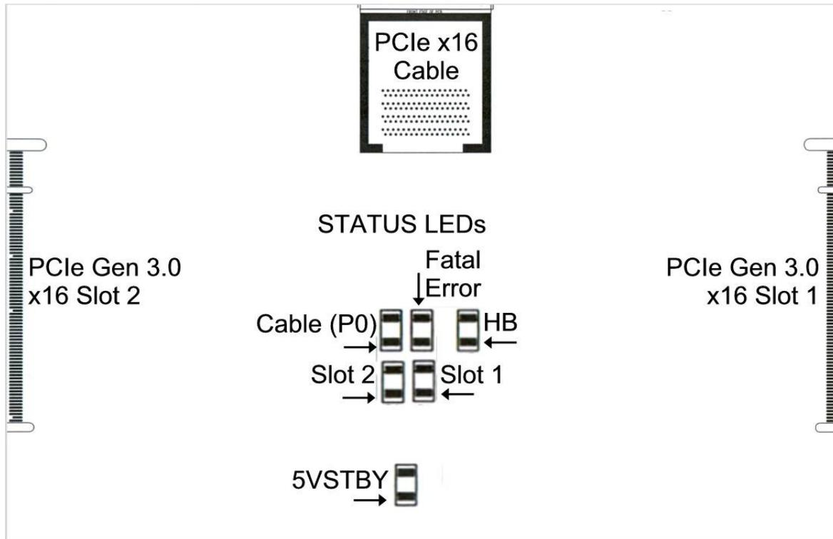
**Xpander is functioning properly once the Cable LED (P0) lights green. Proceed to install adapters.**
