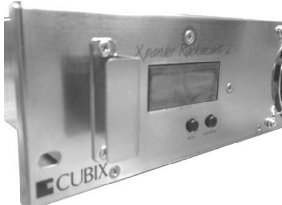
When you first connect power, Xpander comes up in standby mode. The LCD displays Cubix on the top line and Corporation on the bottom line. This is the Start menu. Access all other main menu items by pressing the left button.
