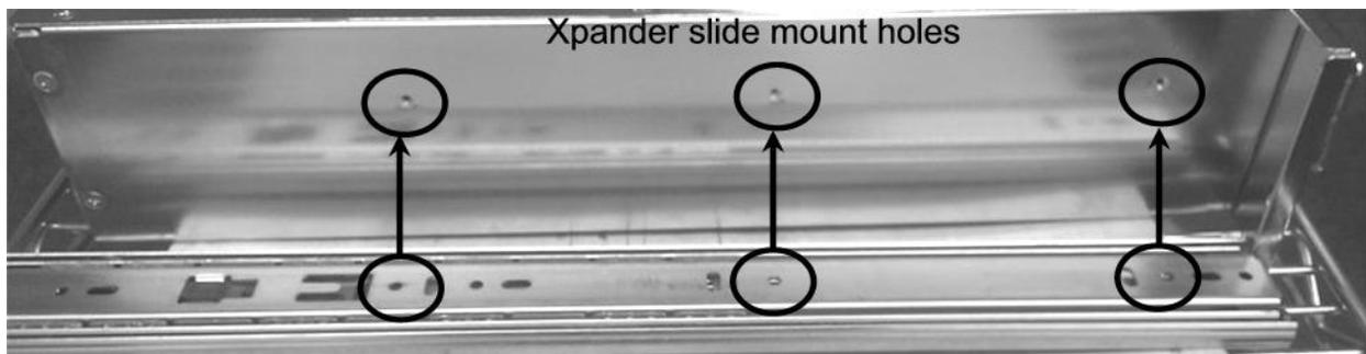
3. Remove the inner slide rail, or slide mount, from the outer rail and mount it to Xpander using the Xpander slide mounting holes. To release each outer slide mount, slide it toward the rear of the enclosure until it stops. Press the catch to release and remove the outer slide mount as you can see in the image at the right.
