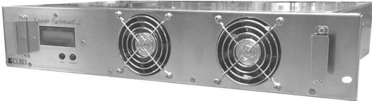
With a HIC installed, a single host computer can support two double-wide graphical processing units (GPUs) inside one Xpander. It connects to one HIC. Rack Mount 2 provides two PCIe Generation 3 (Gen 3) x16 slots for GPUs or other PCIe adapters with multiple Input / Output (I/O) ports such as FireWire, USB 2.0, or high-definition (HD) audio. For example, use NVIDIA Compute Unified Device Architecture (CUDA) -enabled GPUs for rendering, high-performance computing (HPC) or HPC visualization.
